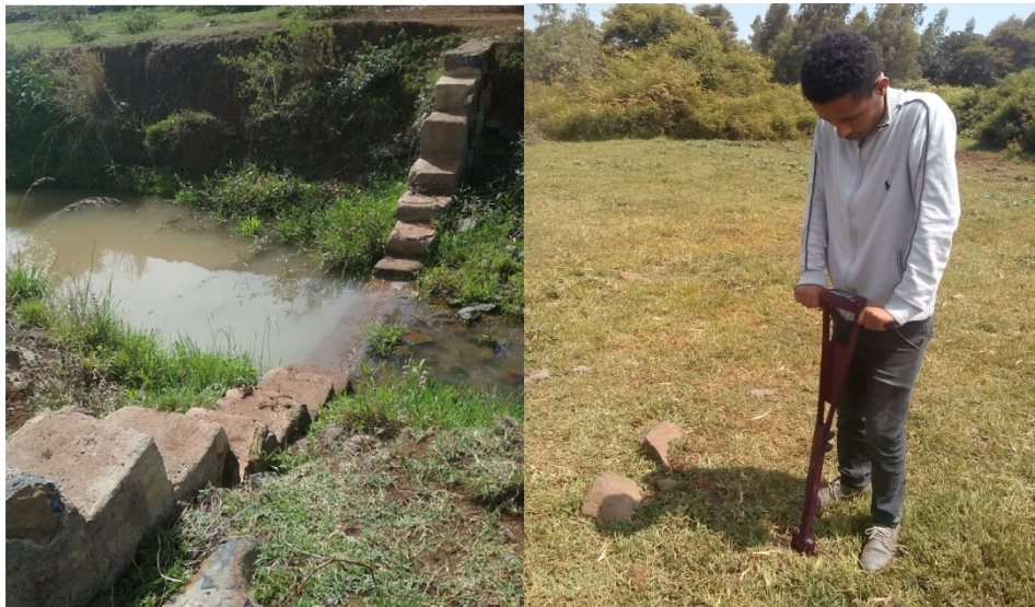
Figure 10 Staff gaging at the out let of Awramba watershed (left) and Soil moisture measurement sites (right)
