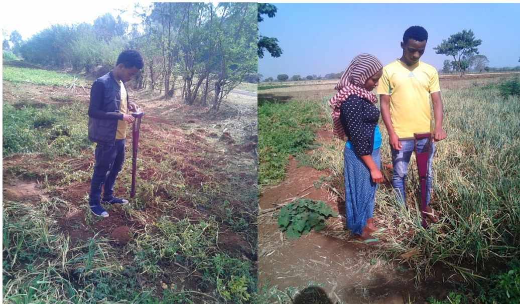
Figure 5 Masters Student (Wondale A.) training about soil moisture data collection using TDR for the high school kids in Koga irrigation site in Chehona command
